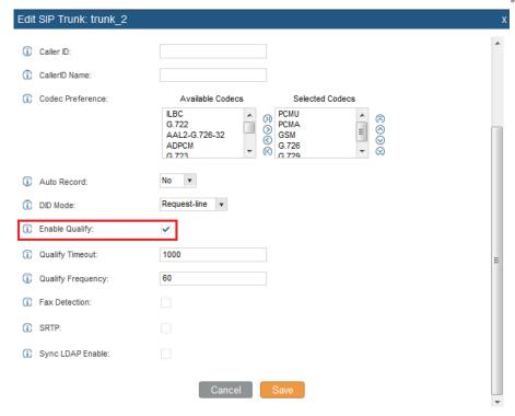
Figure 2: SIP Trunk: Set Enable Qualify
