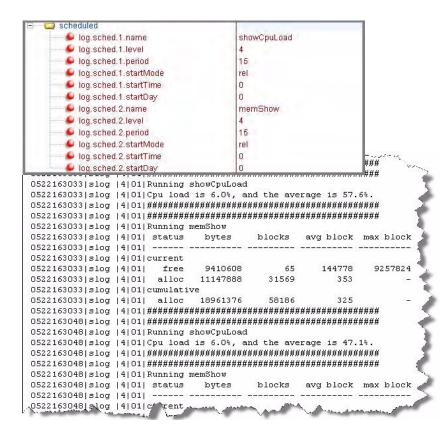
The following figure shows an example of a configuration file and the resulting log file.
