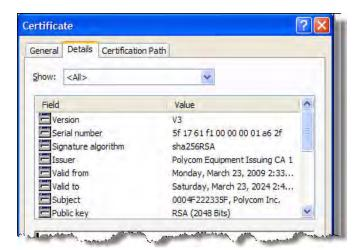
The device certificate and associated private key are stored on the phone in its non-volatile memory as part of the manufacturing process.
