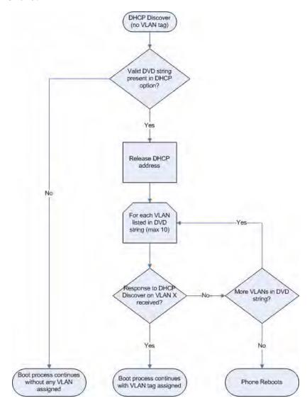
The following figure shows the phone's processing to determine if the VLAN ID is valid:
