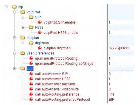
The following example **phone1.cfg** configuration file shows the relevant parameters:
