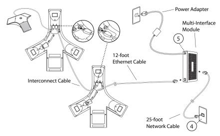
The provisioning over C-Link feature is automatically enabled when a SoundStation IP 7000 phone is not connected to the Ethernet. Both SoundStation IP 7000 phones must be running the same version of the SIP application.
