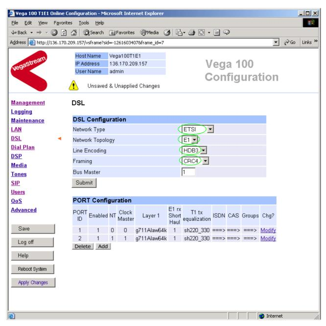
>In the **DSL Configuration** section check that the Network Type = ETSI. *If required QSIG is also an acceptable Network Type for E1 Vega 100s.*
