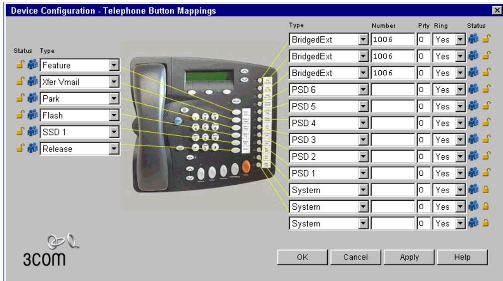
Figure 54 shows a group of three buttons (10, 11, and 12) that have been configured as bridged extension appearances for the extension (1006) associated with the primary telephone.
