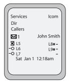
Icons next to the softkeys within the phone's display indicate the status for that line or call and have equivalent status to the line/call appearance lights of the hard keys on the phone. The following table provides a description for each icon.
