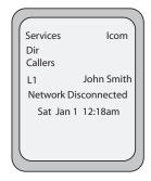
Check that the cables are tightly connected to the phone and to the wall jack. The phone should automatically detect when it is reconnected and dispalys the "**Network Connected**" prompt for a few seconds. However, if changes have been made to your phone's network settings, you may need to restart your phone.
