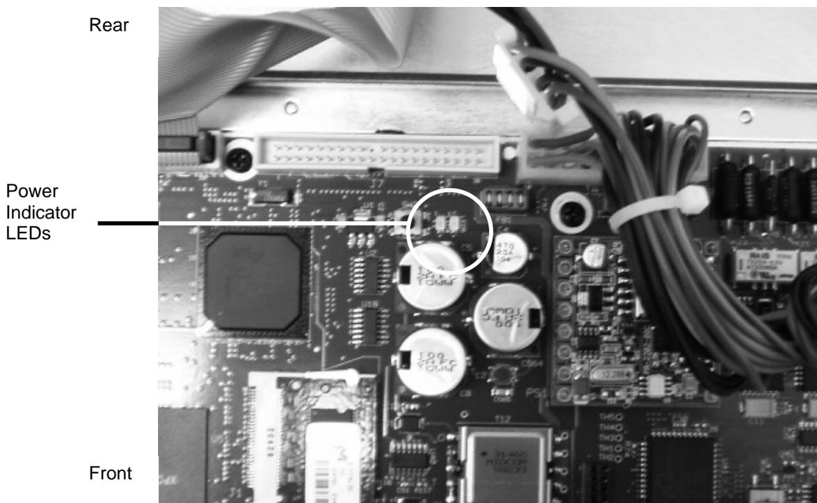
Figure 3: Motherboard Power Indicator LEDs
