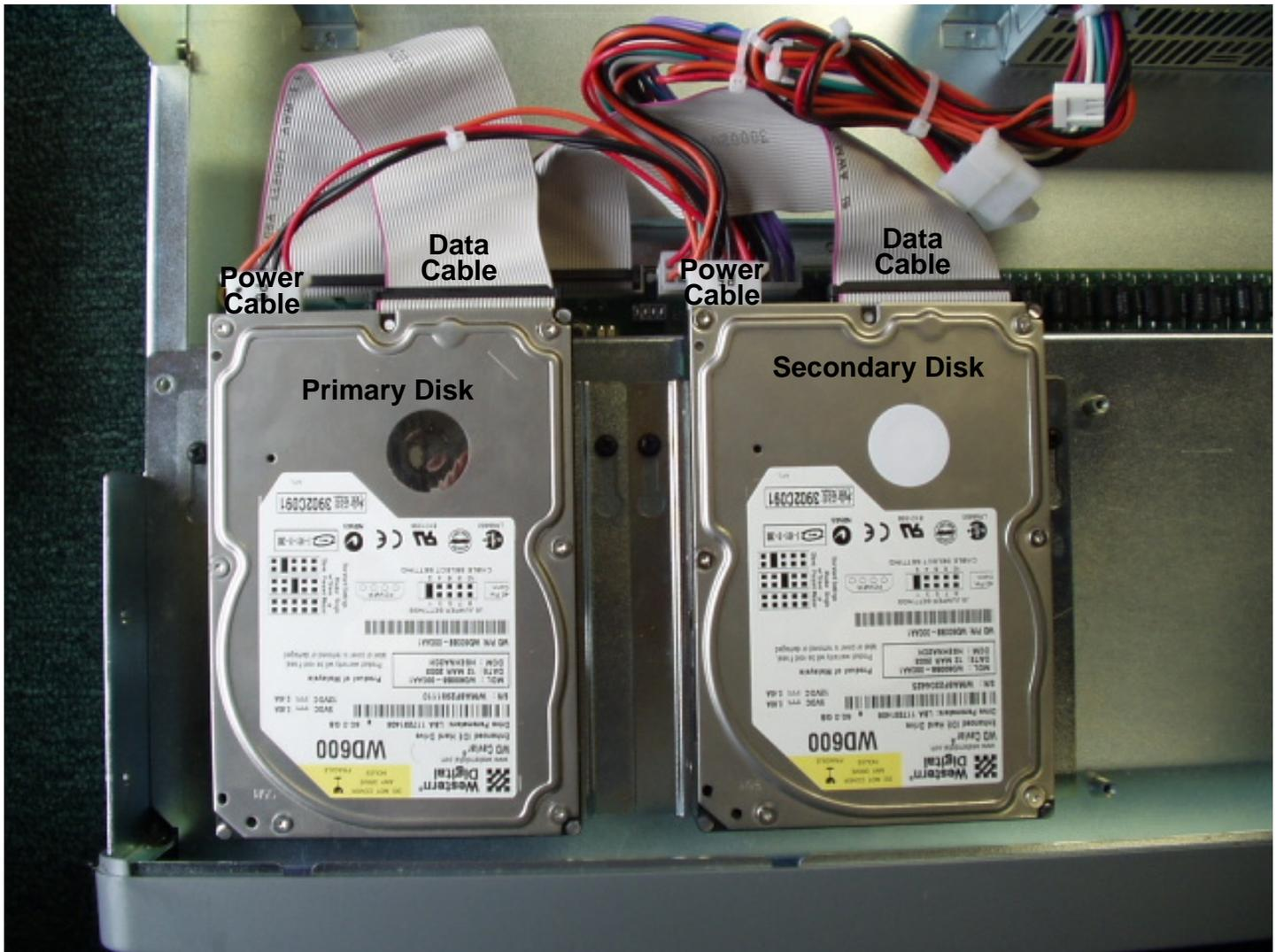
Figure 4 - Disk Positions and Cabling
