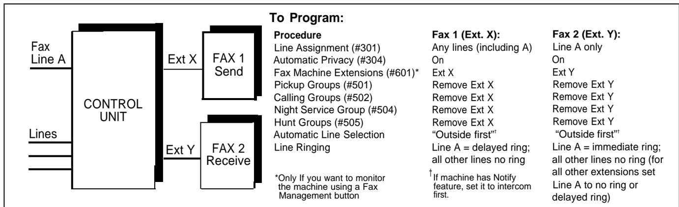
**Figure 5-3. Send and Receive Fax Machines**
