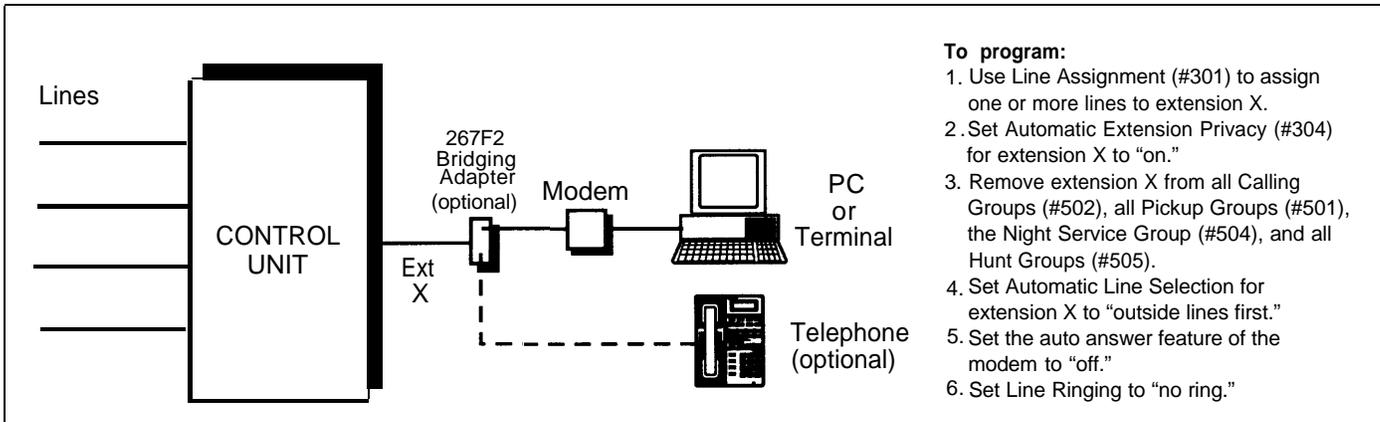
**Figure 5-7. Stand-Alone Modem for Placing Calls Only**
