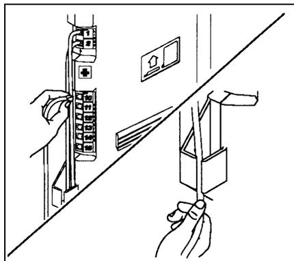
**5** A) Connect modular telephone cords to 206 module extension jacks, starting at the top jack on the leftmost module. B) Route each cord through the hook on the front of the module, then through the slot between the module and the base of the backplane. Leave at least two feet of slack to allow easy replacement of system modules (see "Replacing a System Module" on page 2-12). Connect each cord to the appropriate wall jack.
