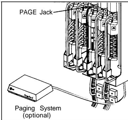
**Paging System:** To install an AT&T paging system, insert the modular plug for the paging system into the jack labeled PAGE on the processor module. Route the cord as for line and extension cords, then connect it to the loudspeaker paging system.
