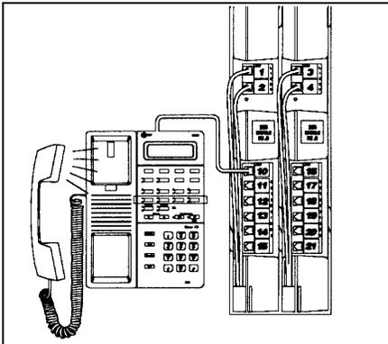
**4** Test the lines. Plug a system phone into extension 10. Press the line buttons for each outside line and listen for dial tone. Repeat for extensions 16, 22, 28, 34, 40, 46, and 52 (if available).
