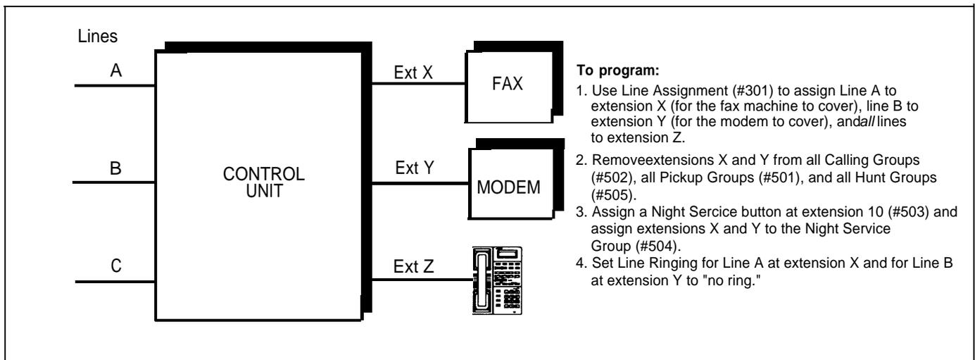
**Figure 5-11. Night Service with Fax Machine and Modem**
