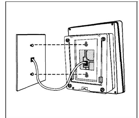
**3** Insert the phone cord through the center of the stand and plug it into the jack on the base of the phone, then plug the other end into the modular wall jack. Mount the phone on the wall jack using the screw keyholes on the base of the stand. For proper mounting, the wall jack must be an AT&T 630B connecting block. Finally, connect the handset cord as described in "Desk Mounting," step 1A above, and label the button sheet as in step 3A above.
