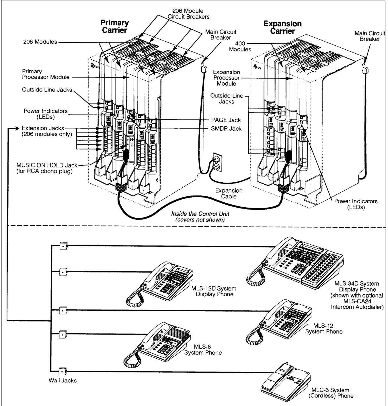
Figure 1-1. System Components
