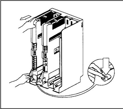
To replace a system module, first disconnect the AC power cord from the wall outlet, and then slide the control unit cover off the backplane.
