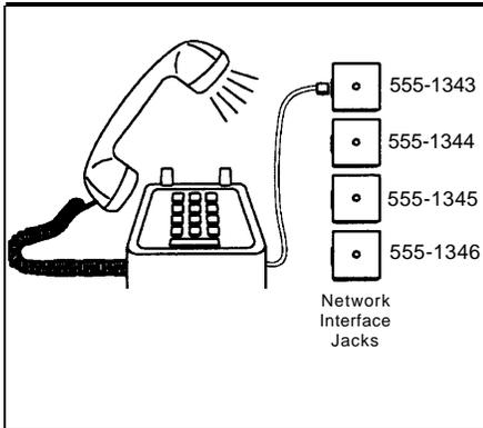
**1** Test for dial tone at the network interface jacks before connecting outside lines. Connect a standard touch-tone or rotary phone to the first network interface jack. Lift the handset and listen for dial tone. Repeat for each network interface jack. (If there is no dial tone, contact your local telephone company before continuing.)
