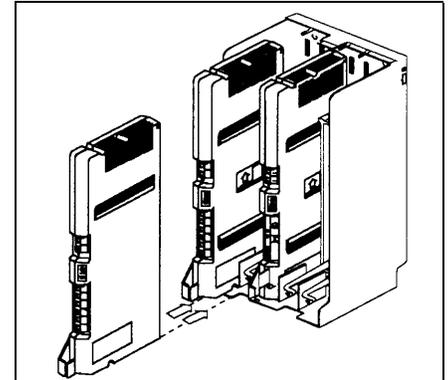
**3** Slide the first 206 module into the *leftmost* slot of the primary carrier backplane. (The system will not work if a 206 module is not installed in this slot.) Going from left to right, install 206 modules first, then any 400 (or 200) modules. The 400 modules *must always* be to the right of all 206 modules, so the extensions will be numbered consecutively.
