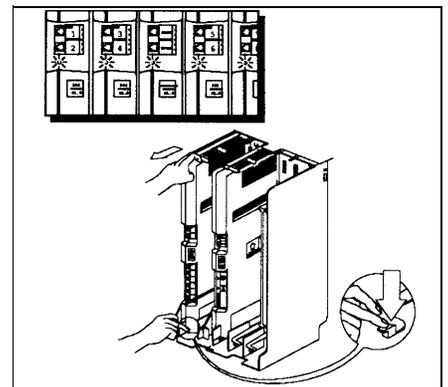
**6** Check all green lights on the fronts of the modules. *If a single light is out*, pull out the circuit breakers, reseal the module, then push in the circuit breakers (as you did in step 5C). *If multiple lights are out*, pull out the circuit breakers, reseal the leftmost module of the ones that are out, then push in the circuit breakers. *If the lights are still out*, call the Helpline.
