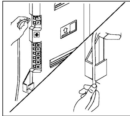
**2** A) Connect telephone cords to the line jacks on 206 and 400 modules, starting with the top line jack on the leftmost 206 module. B) Route each cord through the hook on the front of module, then through the slot between the module and the base of the backplane. Leave at least two feet of slack in the cords so you can easily reconnect cords after replacing system modules (see "Replacing a System Module" on page 2-12).
