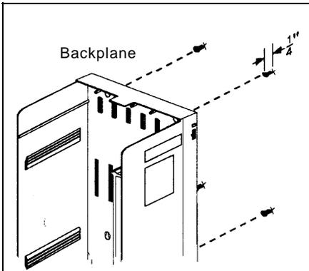
**1** A) Hold the backplane against the wall. (If you are also installing the expansion carrier, plan to install it to the *right* of the primary carrier, leaving 6" to 24" between carriers.) Using the four screw keyholes in the backplane as a template, mark screw locations on the wall. Start four #12 screws, leaving the screw heads approximately 1/4" away from the wall. Slip the backplane onto the screws and tighten them. B) If you are mounting the expansion carrier, repeat this step.
