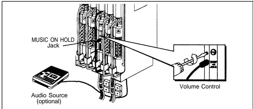
**Music-on-Hold Audio Source:** A) To connect an audio source, insert an RCA phono plug into the MUSIC ON HOLD jack on the primary processor module. Route the cord as you did for line and extension cords, and then connect it to the audio source.
