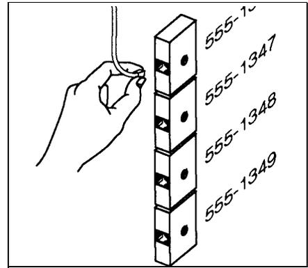
**3** Connect the free end of each line cord to the appropriate network interface jack.
