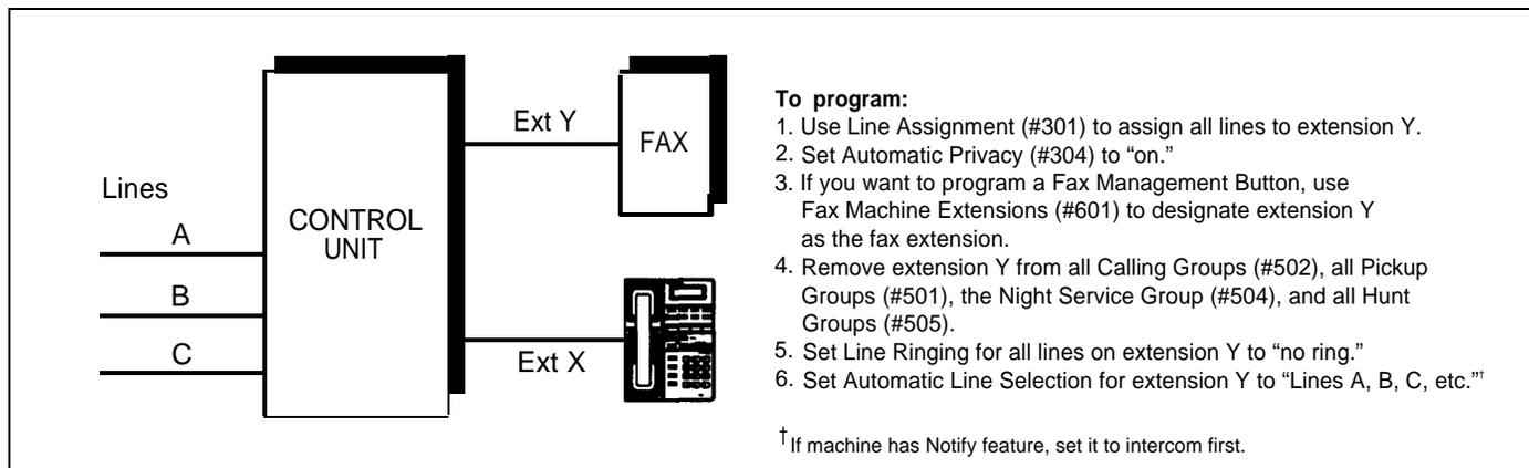
**Figure 5-2. Fax Line Saver Setup**
