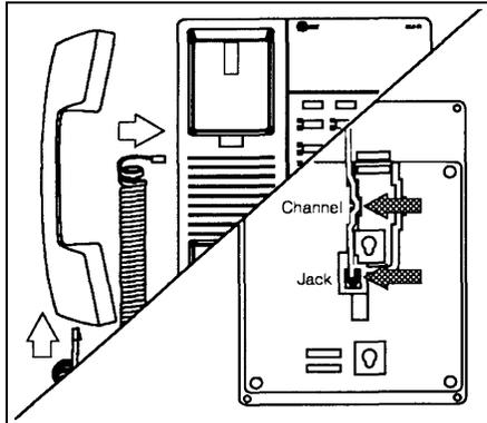
**1** A) Plug one end of the handset cord into the jack on the handset and the other end into the small jack on the left side of the base. If installing an MLS-34D, go directly to step 2 (skip 1B). B) Plug one end of the phone cord into the big jack on the bottom of the phone. Push the cord into place along the channel on the bottom of the phone. If you want to raise the angle of the phone, go to step 2 and install the telephone stand. If not, go to step 3.
