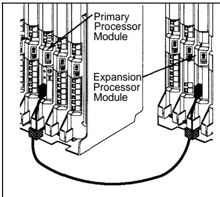
**4** If you have installed both carriers, plug the ends of the expansion cable into the two processor modules and tighten the screws. Route both ends of the cable through the hooks on the fronts of the modules.
