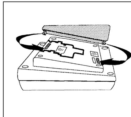
**2** To install the telephone stand, gently place the phone upside down with the low end of the phone to your right. Insert the tab on the narrow end of the stand into the left slot on the bottom of the phone. (For an MLS-34D phone, feed the cord through the stand and plug it in.) Then insert the other tab into the right slot, pushing the stand down and slightly inward until the tab locks into place.
