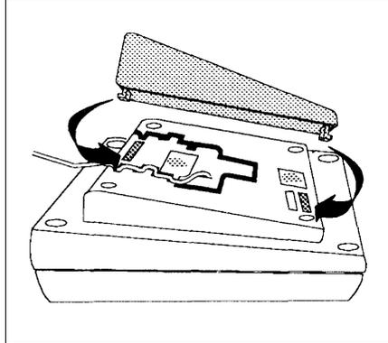
**2** To install the telephone stand (required for the MLS-34D), gently place the phone upside down, with the low end of the phone to your right. Insert the tab on the narrow end of the stand into the right slot on the bottom of the phone. (For an MLS-34D phone, feed the cord through the stand and plug it in.) Then insert the other tab into the left slot, pushing the stand down and slightly inward until the tab locks into place.
