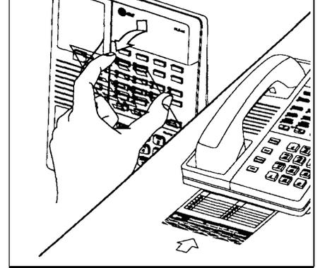
**3** A) Remove the plastic cover from the phone and place a labeled button sheet on the phone so the holes on the sheet fit over the buttons. Carefully replace the plastic cover. B) Slide the *Quick Reference* card under the telephone.
