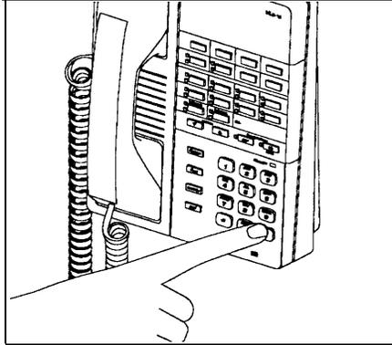
**2** Test the telephone for proper operation. To test the power and lights on a system phone, press and hold the [#] button for five seconds. Before releasing the [#] button, lift the handset. All lights should light, the ringer should sound, and (on the MLS-12D or MLS-34D phones only) a test pattern should appear on the display. (If not, call the Helpline at 1 800 628-2388.) Replace the handset; the phone is now in normal operating mode.
