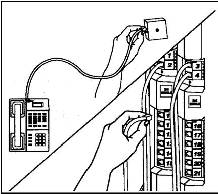
**1** To connect a phone, plug the modular telephone mounting cord into a modular wall jack or directly into a 206 module extension jack. (If you are connecting a standard phone and its mounting cord is loose, use an AT&T D2R mounting cord instead.)
