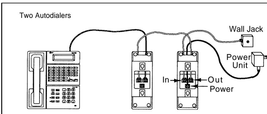
**1** To wire two Intercom Autodialers to a system phone: A) Connect the phone to the first autodialer, following the instructions in step 1A above (the figure at the top of this page). B) Using the second D8W cord, connect the two autodialers together: plug one end of the line cord into the IN jack on the first autodialer, and plug the other end into the OUT jack on the second autodialer.
