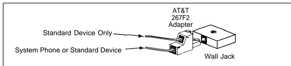
**Figure 2-2. Connecting Two Devices on One Extension**
