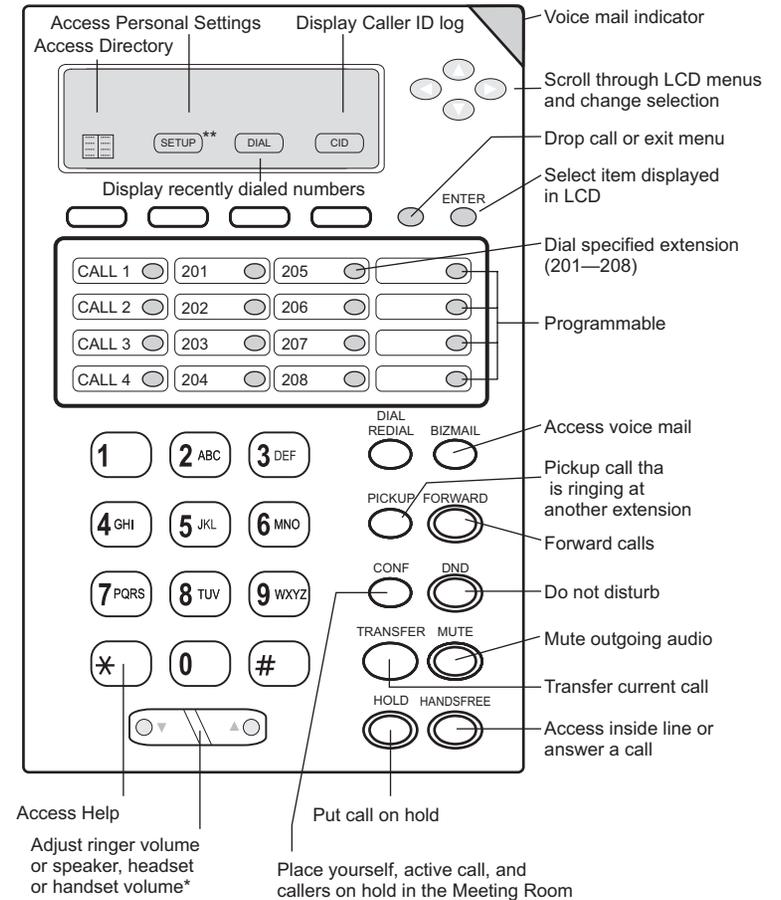
\*When you are not on a call, the buttons adjust the ringer volume. When you are on a call, the buttons adjust the volume of the handset, speaker, or headset.
