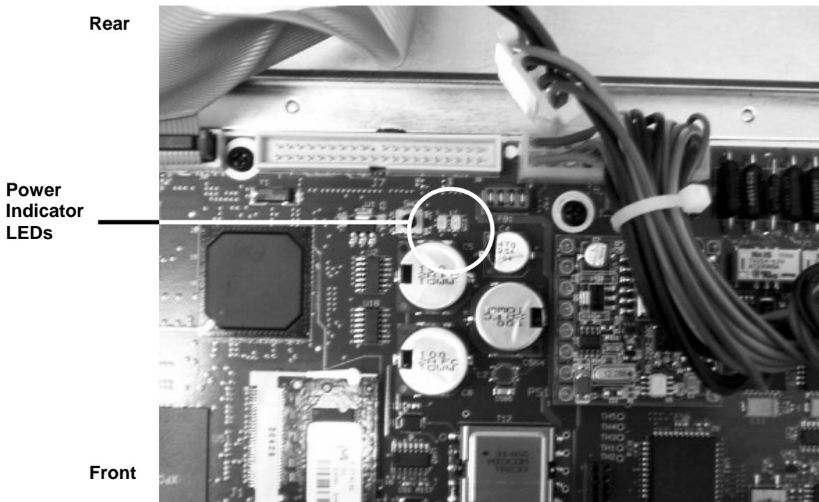
Figure 3: Motherboard Power Indicator LEDs
