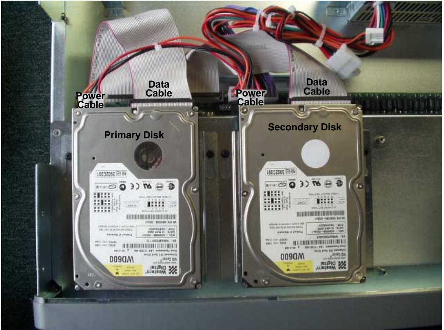
Figure 4 - Disk Positions and Cabling
