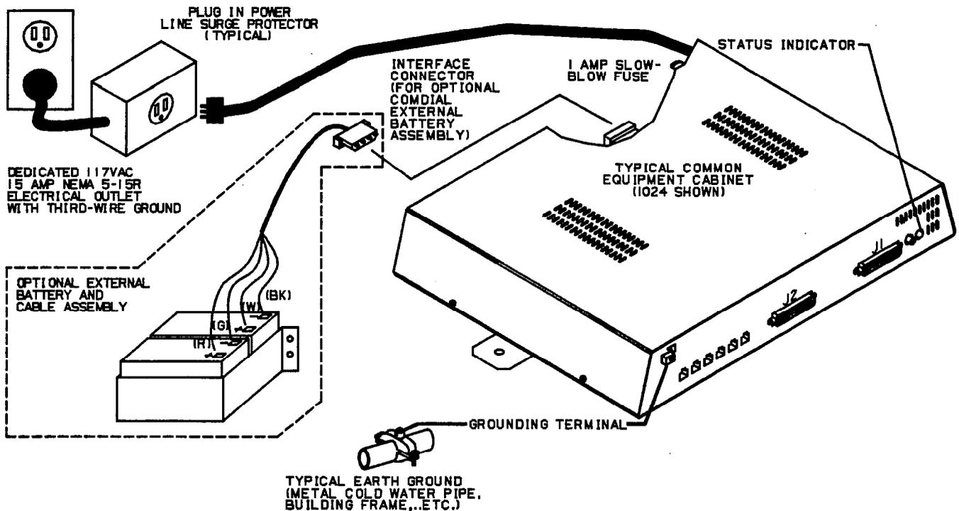
Figure 3-2. AC Power Connection and System Grounding
