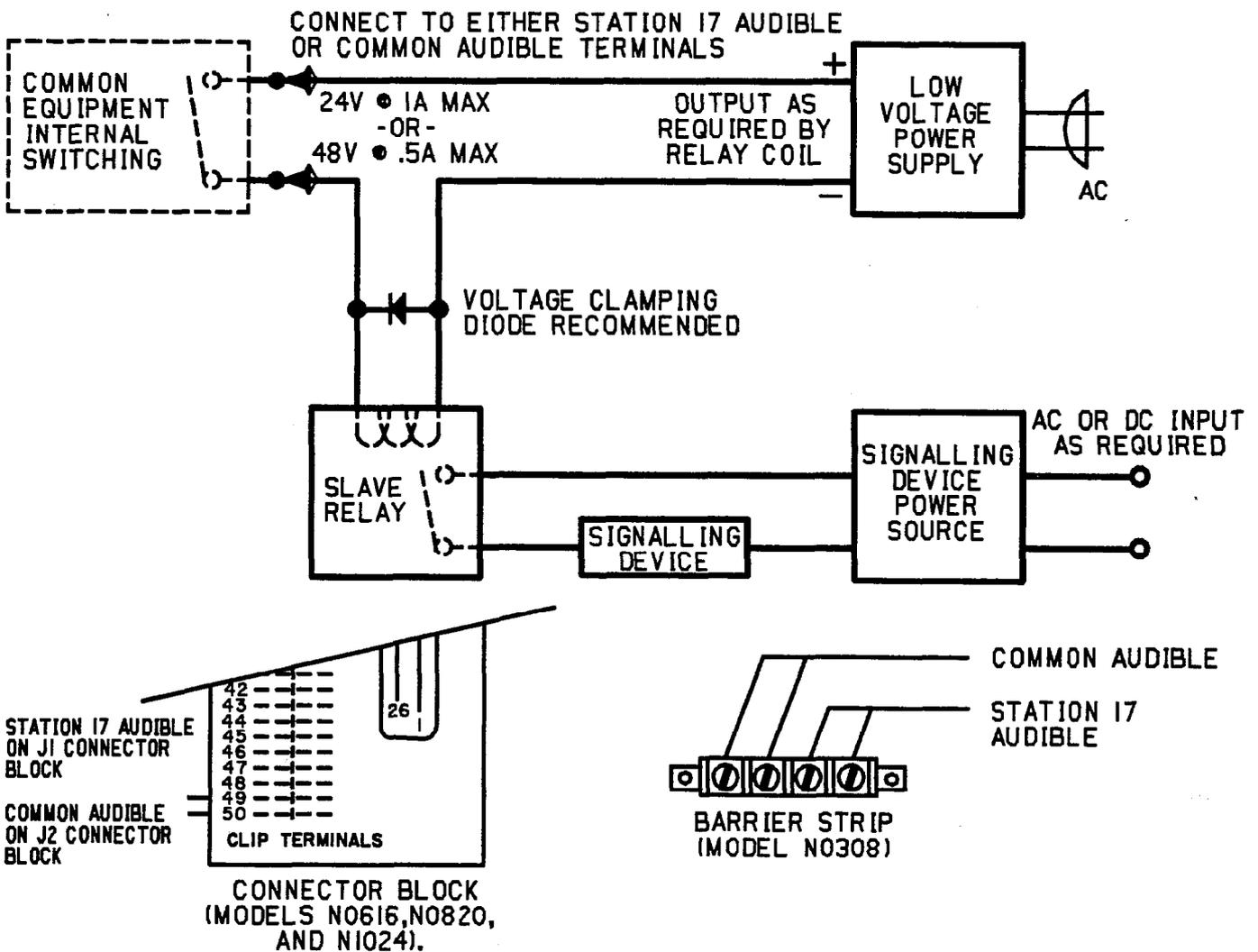
Figure 3-6. Common Audible and Auxiliary Station Interface
