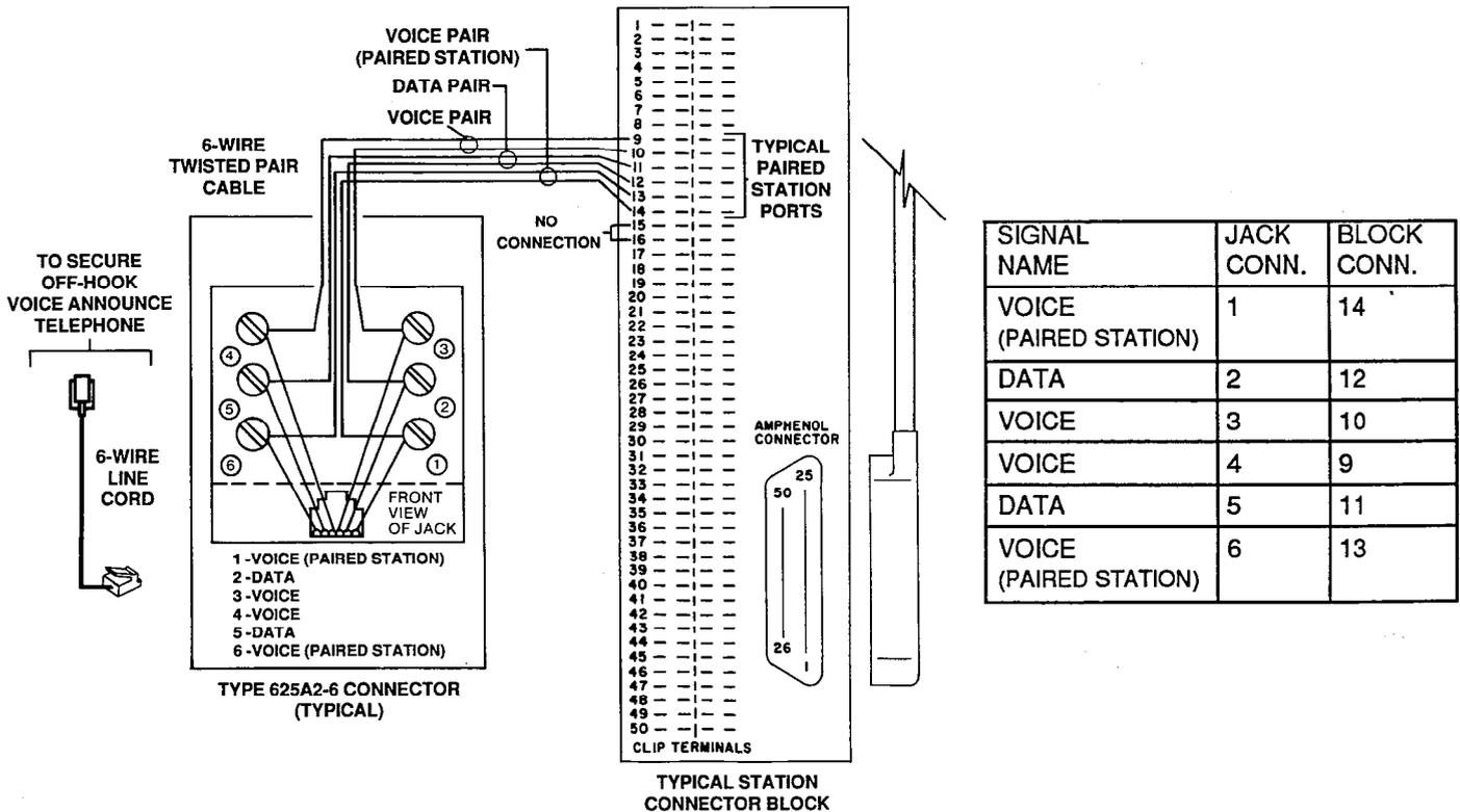
Figure 3-4 Secure Off-Hook Voice Announce Connections
