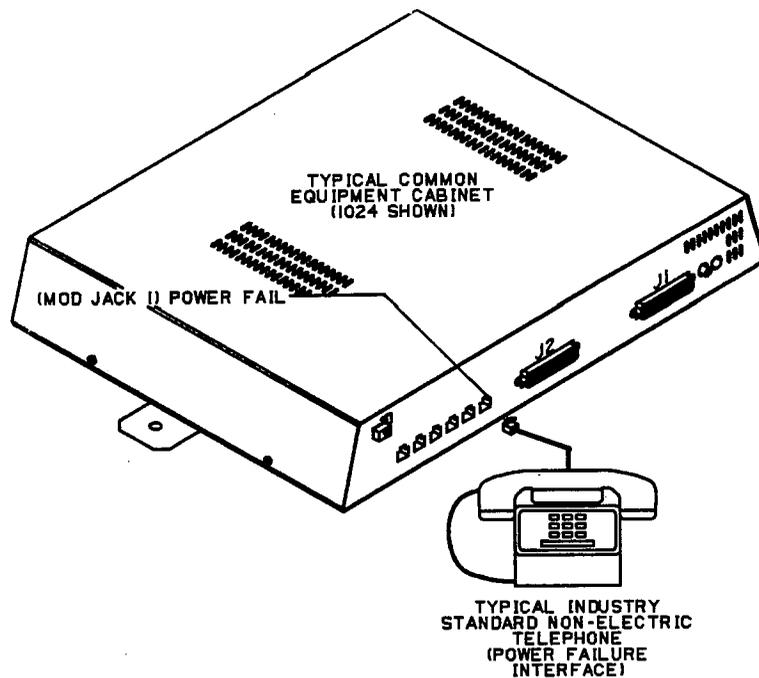
Figure 3-5. Power Failure Station Connection.
