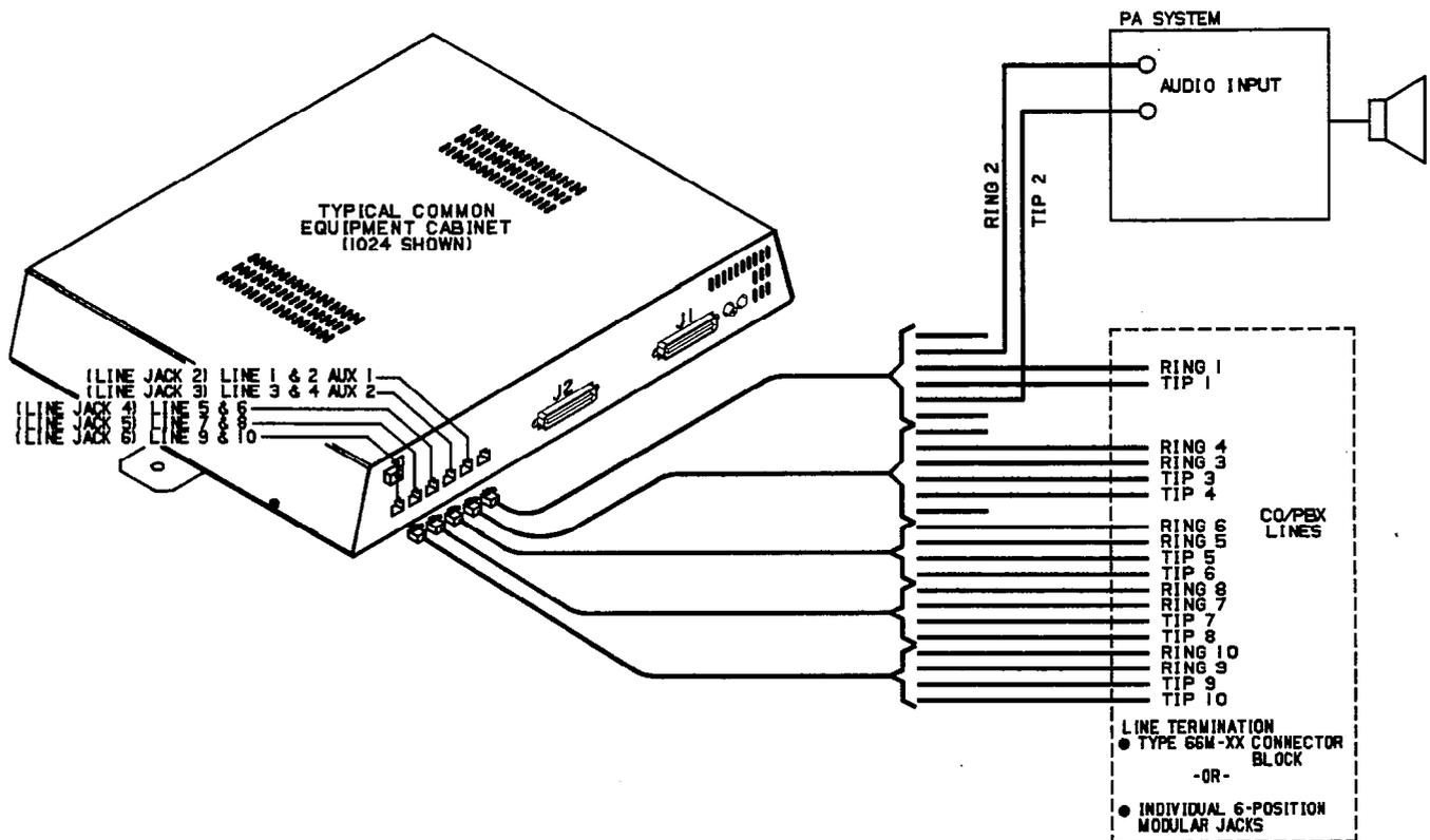
Figure 3-8. External Paging Interface - Line Port
