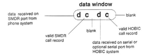
Watch the data window as you make your HOBIC test calls. As the PL receives call records from the HOBIC system on the serial or optional serial port, a "d" flashes in the fourth space (see diagram above) of the data window. A "c" flashes next to the "d" when the PL determines the call is valid.
