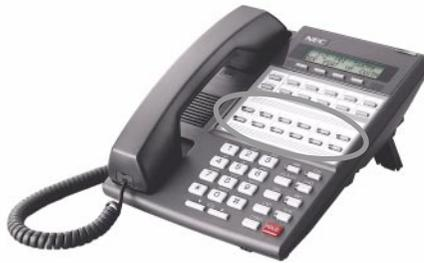
The **22-Button Standard and Display Telephones** feature 12 Programmable Function Keys.
