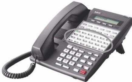
The **34-Button Display Telephone** features 24 Programmable Function Keys.
