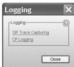
2. Select the *SIP Trace Capturing* url to open a browser interface to permit detailed logging of SIP messages for calls to IP phones and/or VoIP lines.
