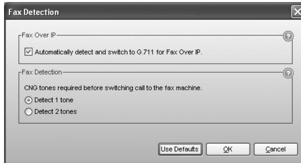
2. Select the *Automatically detect and switch to G.711 for fax over IP* checkbox to have the unit detect fax over IP and then switch to G.711.
