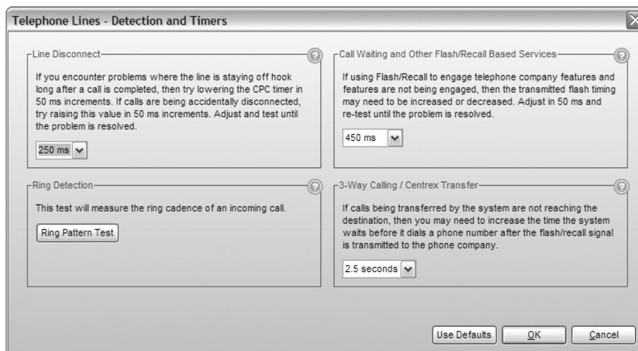
The *Line Disconnect* timer controls the duration a telephone line may be disconnected before the system clears the telephone call. In some cases this may be used by the telephone network to indicate a calling party has hung up and the call has ended (also known as Disconnect Clear, K-Clear or CPC signal). Incidents of disconnected calls may indicate a faulty telephone line, or may be resolved with a longer *Line disconnect* time setting.
