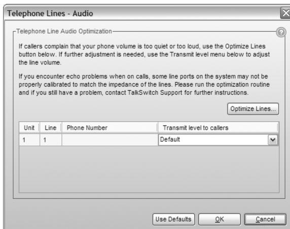
2. Optimize the unit to match the far end impedance of the telephone lines. Click *Optimize Lines*. The *Optimize Lines* window appears. Click *Run Optimization*.
