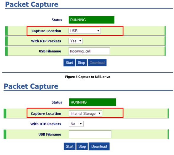
Figure 9 Capture to internal storage
