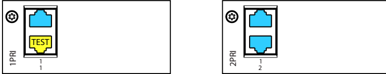
Fig. 39 Connection possibilities for PRI network interfaces
