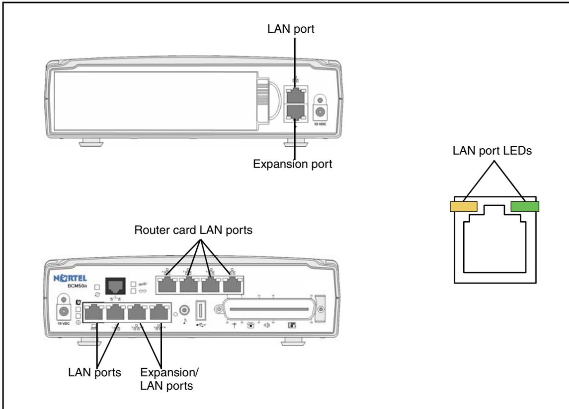
The table [LAN port and expansion port LED indicators](#) on page 20 describes the possible LED states for the LAN ports LEDs.
