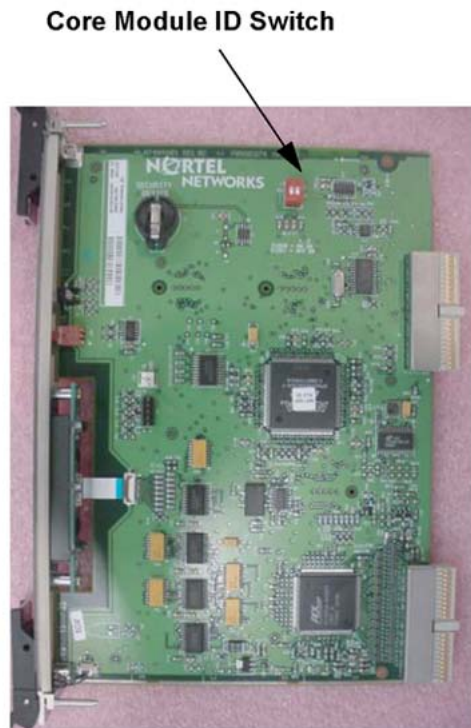
Figure 7 Core Module ID switch
