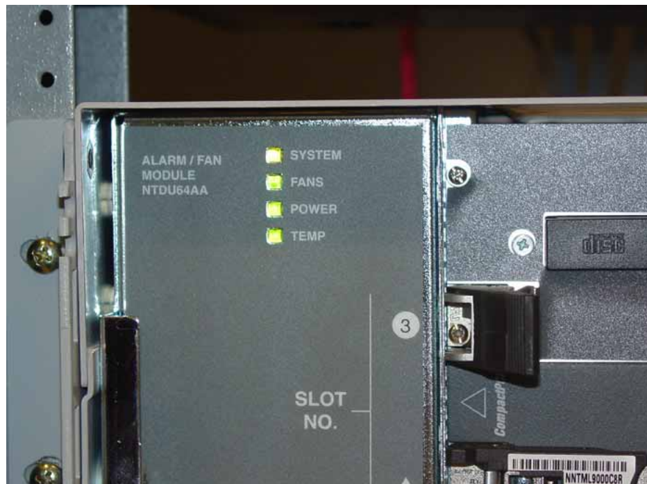
Figure 2 Alarm/fan module status LEDs
