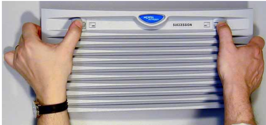
Figure 48 Depressing latches and pulling back on front cover
