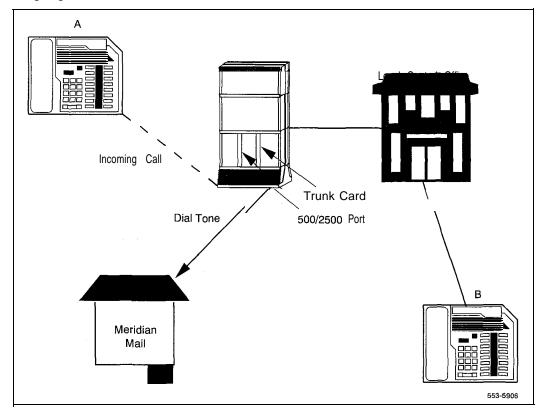
This illustration shows an outgoing call to from the Meridian 1 system to the Central Office. Station A transfers Station B to Meridian Mail and goes on-hook. The dialtone is provided by the 500/2500 type port with the new CLS LDTA after Station B disconnects.
