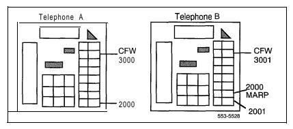
CFW DN on Telephone A is DN 3000. CFW DN on Telephone B is DN 3001.
