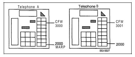
CFW DN on Telephone A is DN 3000. CFW DN on Telephone B is DN 3001.
