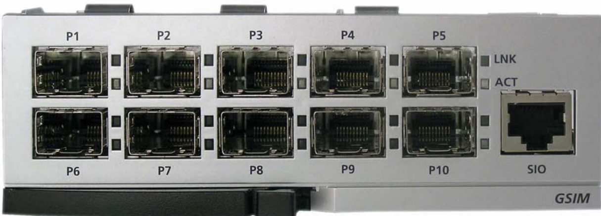
Figure 3.38 Front View of GSIM Module
