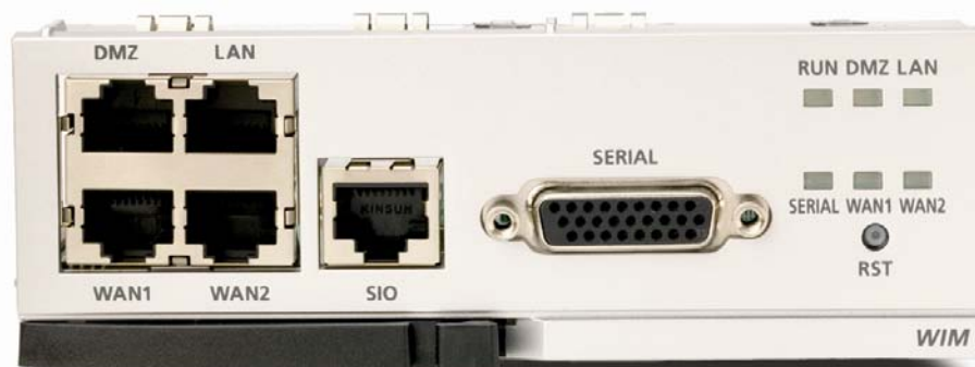
Figure 3.25 Front View of the WIM Board
