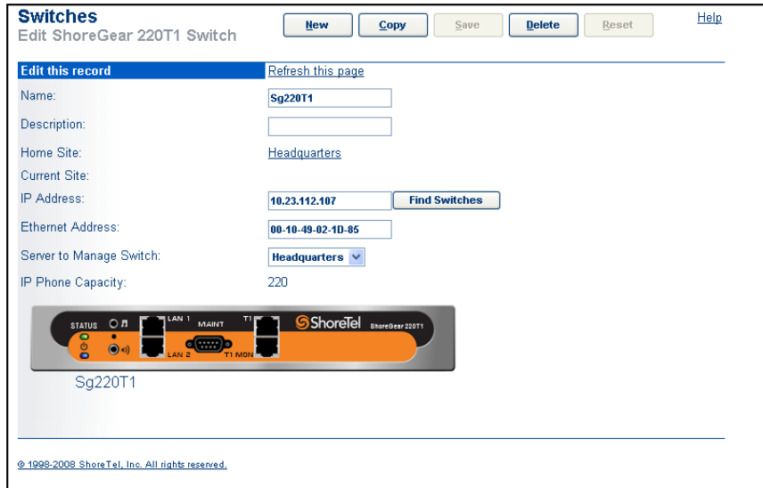
Figure 5-12 Edit Spare Switch panel
