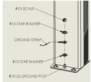
No more than 15 units may be grounded through one connection to the protective earth ground. Systems involving more than 15 units must be broken up into groups of 15 or fewer units with each group provided with an independent protective earthing conductor.
