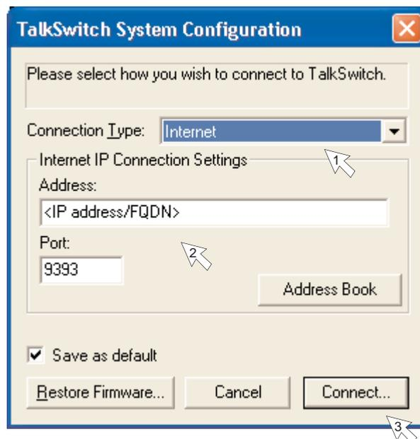
**OBTAINING THE IP ADDRESS OF A REMOTE TALKSWITCH 48-CVA**
