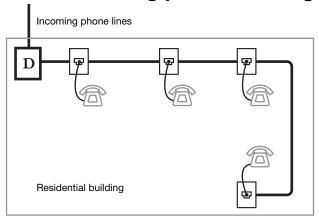
All phones are connected together in a single loop (or in multiple loops).
