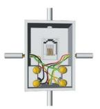
The demarcation point is the point of interconnection between the telephone company facilities and your building.
