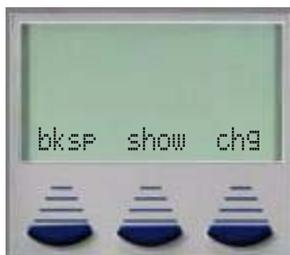
This screen allows the programmer to enter a MBC and then Press **show** and jump directly to the programming parameter. For example to set the System Time and Date enter 415, the display will show 4-15, and then press **show**.
