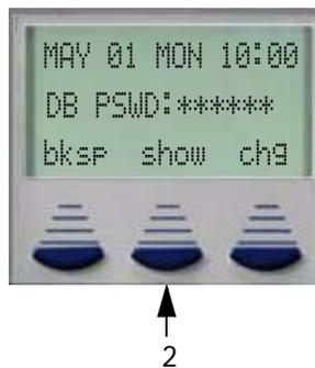
The initial display, which appears to be blank is the **Menu Bypass Code (MBC)** Entry screen.
