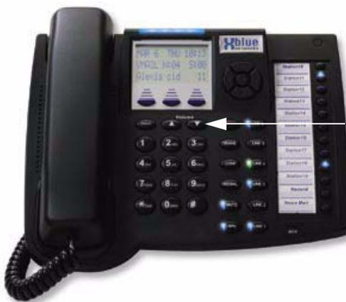
Press the **Volume Up** or **Volume Down** To reenter the **MBC Input Screen**
