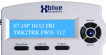
Trunk to Trunk Forwarding
