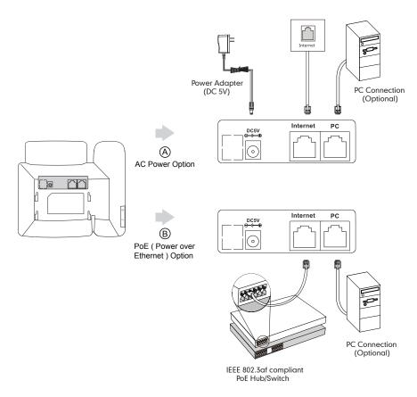
**Note:** PoE is only applicable to the SIP-T20P IP phone. If inline power (PoE) is provided, you do not need to connect the power adapter. Make sure the Ethernet cable and hub/switch are PoE compliant.
